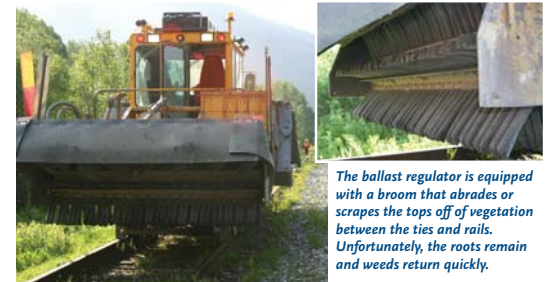
A rail-mounted brush cutter provides one method of mechanical vegetation control.
