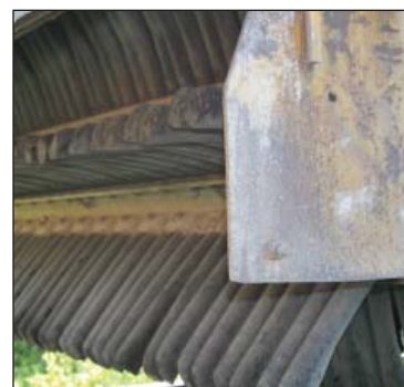
Above and right: The ballast regulator's bristles are normally covered with rubber. The rubber is stripped to expose the wire when the ballast regulator is used for vegetation management.
