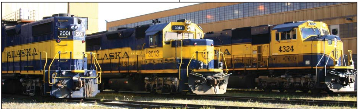
Left to Right: GP-38 locomotive (No. 2001), GP 40-2 locomotive (No. 3013) and SD70MAC locomotive (No. 4324).
